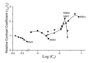
Fig. 4 Effects of inhibitors at different concentrations on relative contrast coefficients
