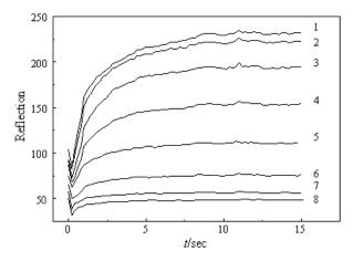
Fig.2 the relationship of reflection light intensities and time in different exposed level with CCD exposure Increased with sequence 1 to 8
