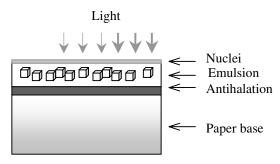
Fig. 1 Cross section of CTP printing plate
